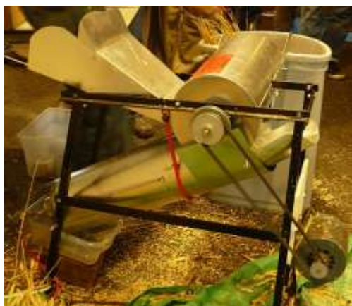
A thresher/winnower for dry beans and small grains, built by John Howe of Waterford, Maine.
