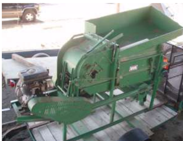
Stationary thresher used to clean grain in the field.
